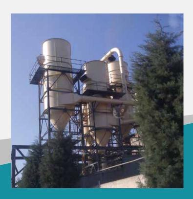
Cylindrical filters are manufactured with ordinary or anti-static bags up to a capacity of 120 m2 including dust filtration capability for high vacuum or explosion. They are particularly used in coal, wood, food and chemistry industries.
