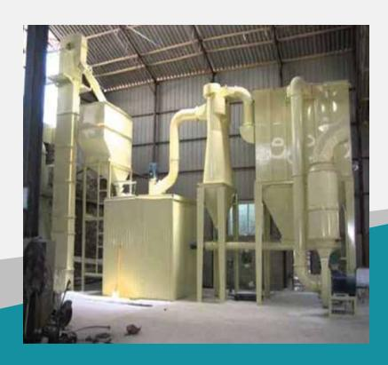
They have a compact structure. They are provided with polyester or net bags. They are used in hopper-top discharging, conveyor band discharging, point dust elimination operations. They are produced up to a capacity of 32 m2 with a full-accessory fan or fanless.
